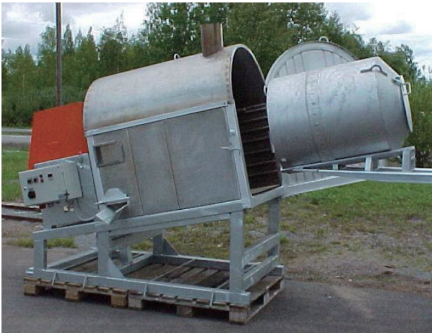
Figure 3 Dross Processing Furnace (patented) 14)
