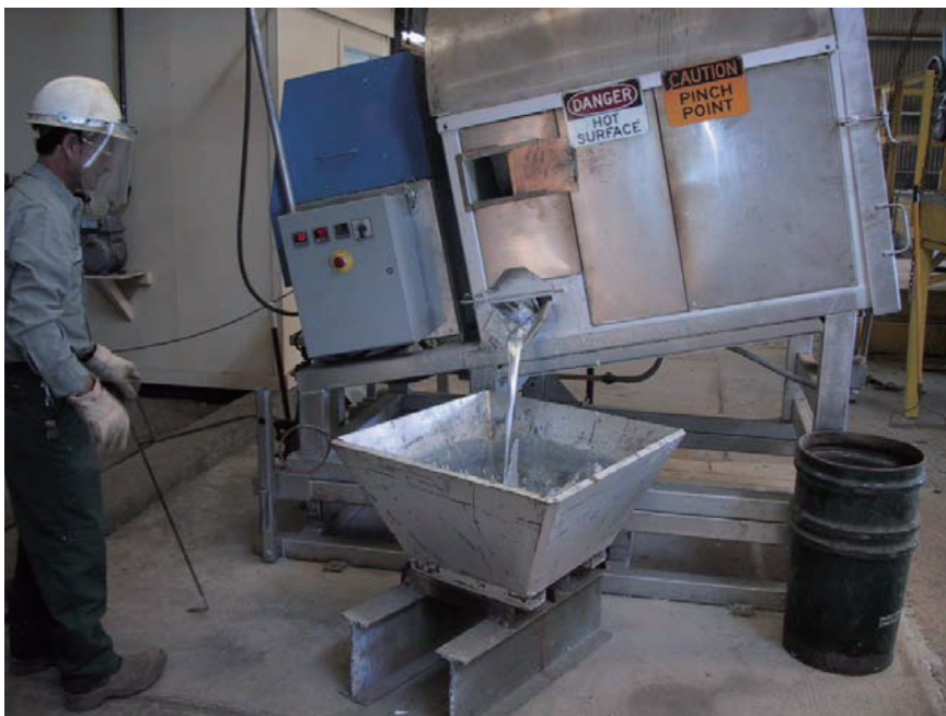
Figure 4 Pouring Recovered Zinc from Galvanizing Dross 15)
