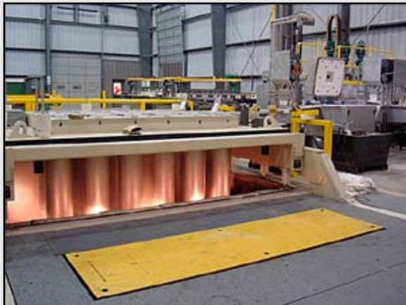
The SNIF SHEER® P-180UiT is a triple rotor degassing system capable of treating high volumes of molten aluminium. Immersion heaters are used to maintain metal temperature during casting and the SHEER nozzles provide highly efficient hydrogen removal from molten aluminium, resulting in improved metal quality. Lower hydrogen levels mean lower porosity in the finished billet.
