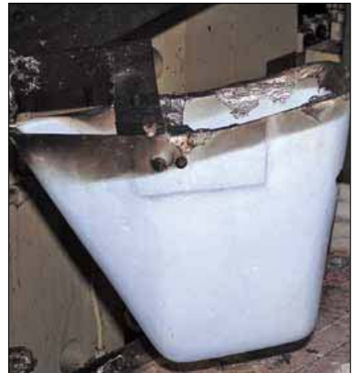
Shown is a 12-lb. reinforced fiberglass material ladle with a non-wetting boron nitride coating.
