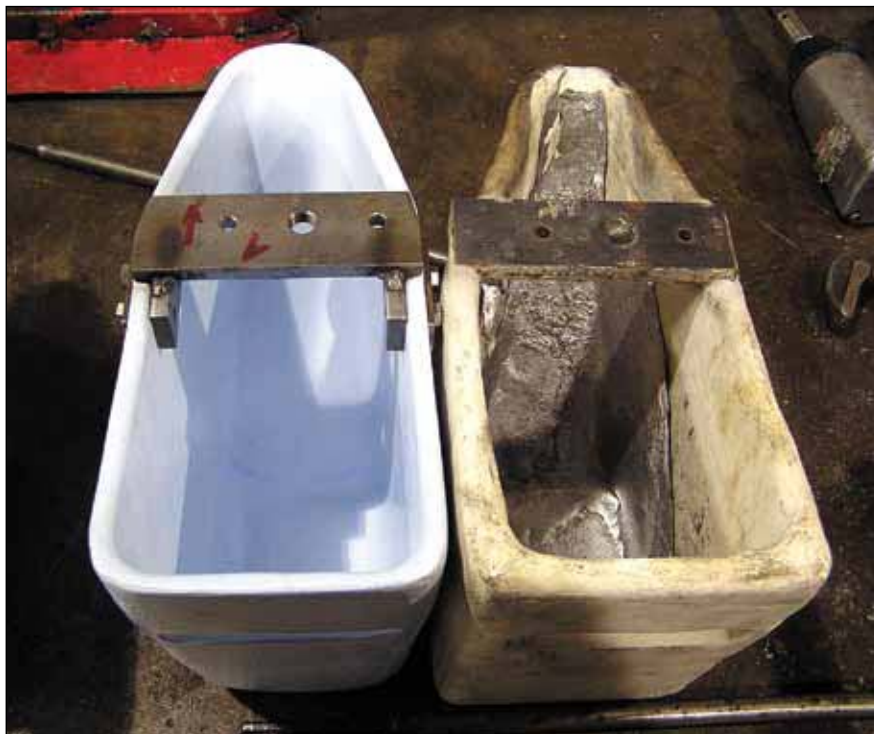
Reinforced fiberglass material ladles (left) routinely have service life of six months, compared to two to six weeks of service with fiber laminate ladles.
