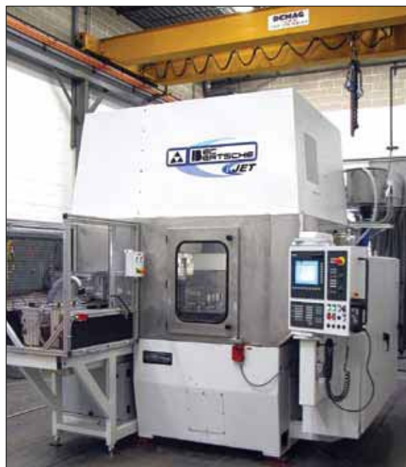
The Bertsche 4-axis iJet with integral drying station and post deburr/part rinse station is a hybrid of mechanical deburring and high pressure water deburring.
