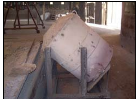
View of MZR Drum at the side of the kettle; ashes are directly transferred from the kettle into the drum
