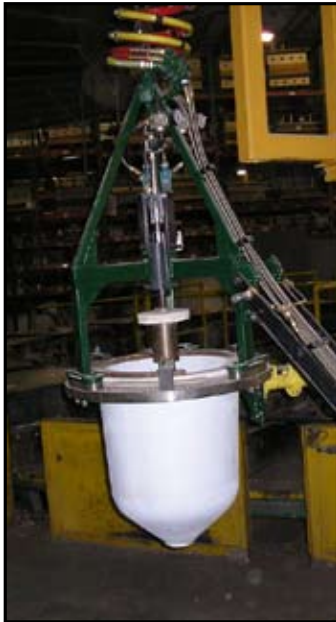
Pyrotek manual bottom-pour ladle system in operation
