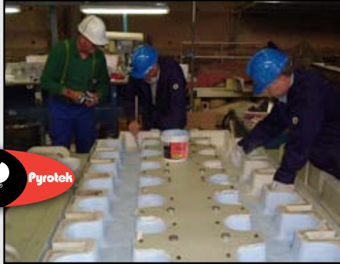
BN coatings applied to refractory of molten aluminium delivery system
